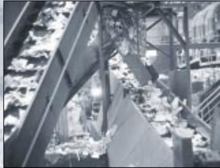
Conveyor belts carry recyclable materials to the sort line where they will be separated.
