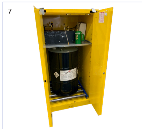
1 - Simple Green, 2 - Reusable bulk aerosol canister, 3 - Aerosol brake cleaner, 4 - CRC Smartwash, 5 - Ozy Juice, 6 - Ultrasonic parts washer, 7 - Bulk brake cleaner systems, 8 - Inland Technology Breakthrough® Product & Parts Washer
