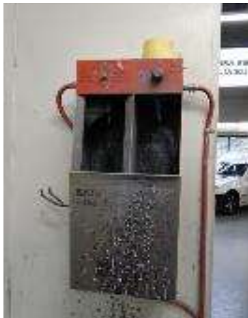
Figure 2 Pneumatic waterborne gun cleaning system
