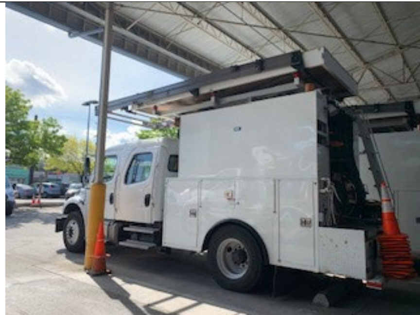
Fiberglass floored platform/lift truck. Safety railings on platform are manually lifted in to place with 50 lbs. of force. Platform is accessed via rear fixed ladder.
