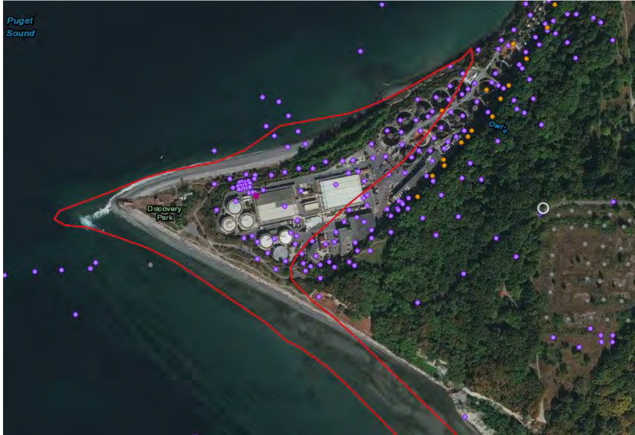
Figure 16: Liquefaction risk zone (red) and boring locations (purple)
