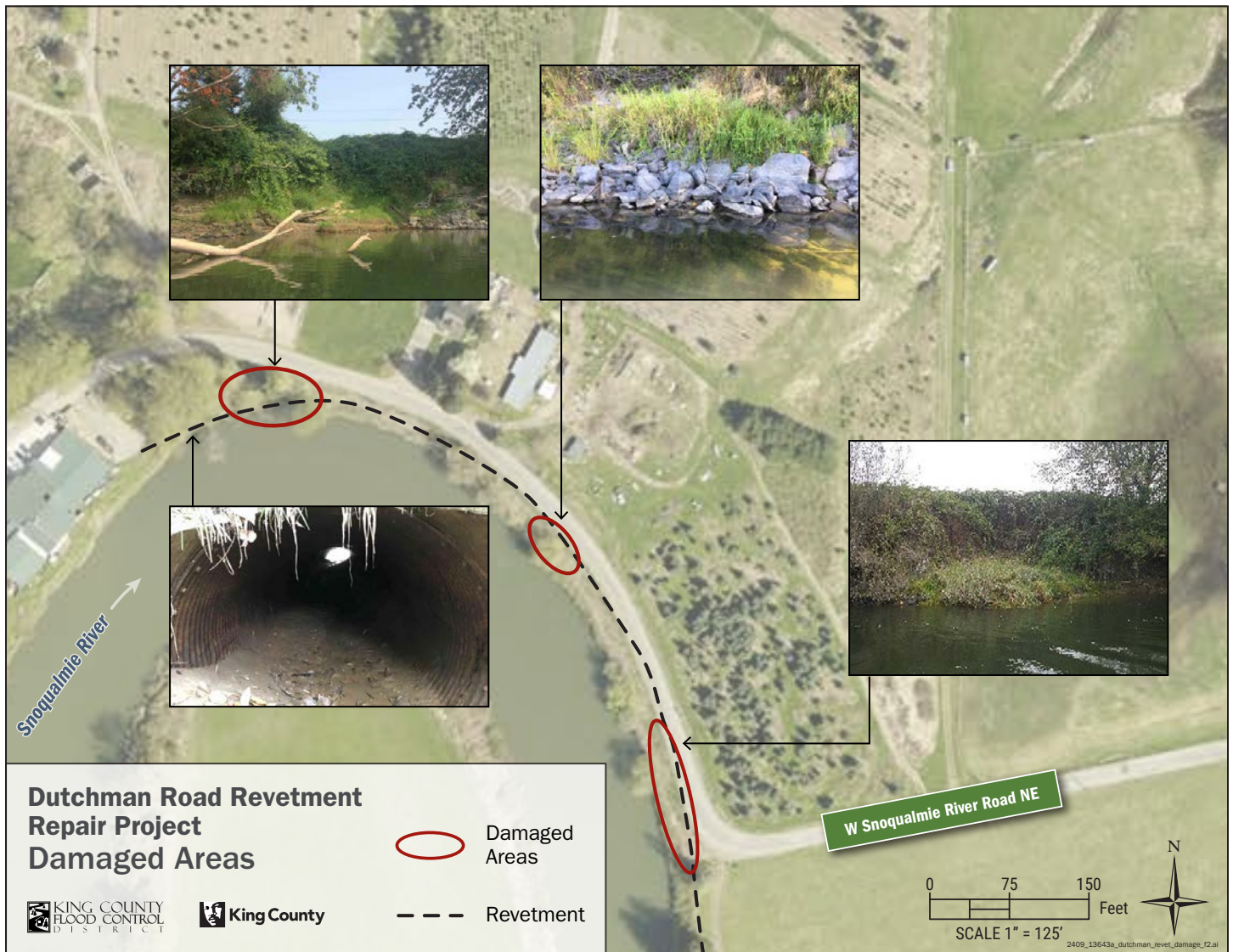
Figure 2. Damages to revetment
