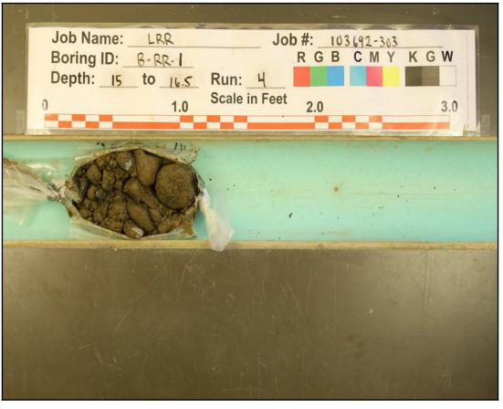
Medium dense, brown to brown-gray, Poorly to Well-Graded Gravel with Silt and Sand and Cobbles (GP-GM/GW-GM) to Poorly Graded Gravel with Sand and Cobbles (GP); moist, wet below about 11 feet; few cobbles; fine to coarse, subangular to rounded gravel; fine to coarse sand; nonplastic. Levee Breach Analysis Mapping and Risk Assessment Geotechnical Data Report King County, Washington
