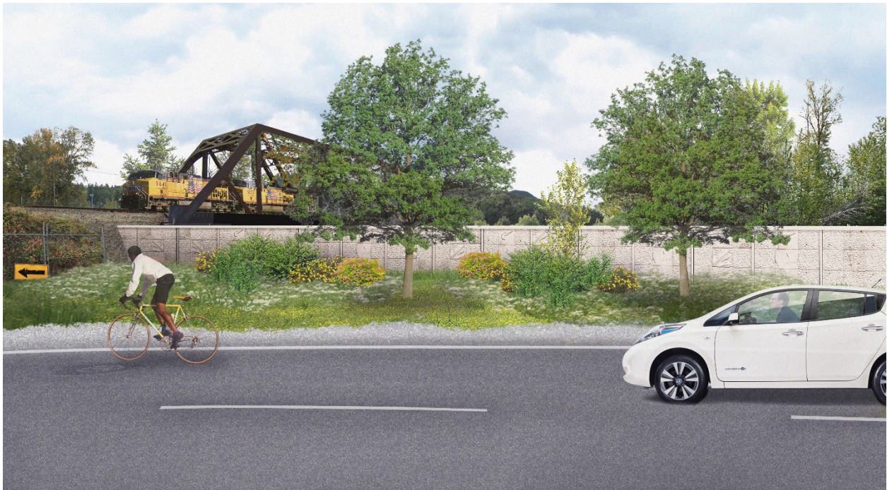
Figure 2-6. Conceptual Depiction of Floodwall Connecting to Existing Railroad Embankment at Third Avenue SE and Skinner Road
