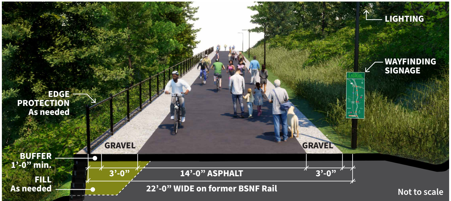
FIGURE 3. TRAIL PROFILE – ON-GRADE TRAIL
