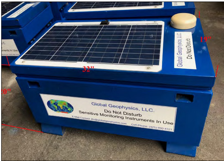
Vibration monitoring equipment will be placed along the trail to monitor vibration during construction activities
