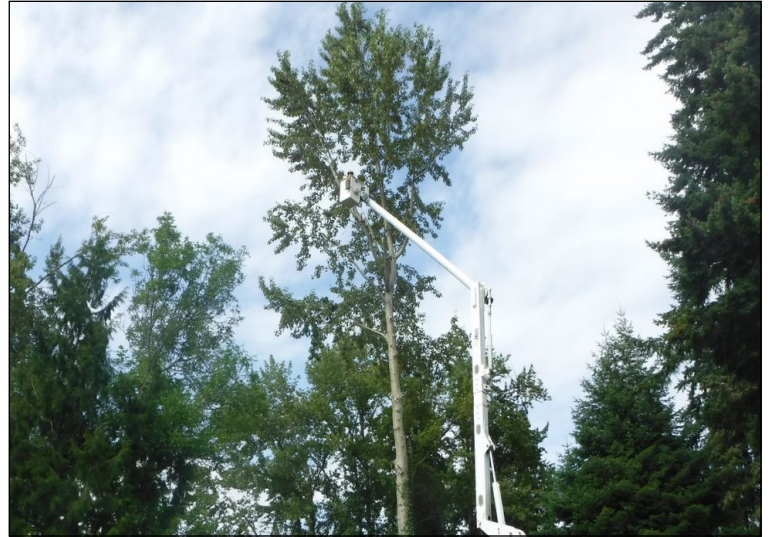
A boom truck is used to remove tall trees, one limb or trunk section at a time.
