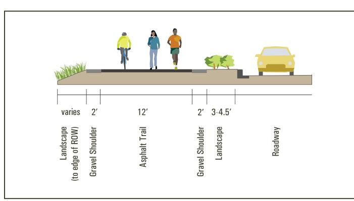
The trail location on the south side of the road will require a few feet of ROW acquisition, eliminate some shrubs lining the road, and eliminate shoulder parking.
