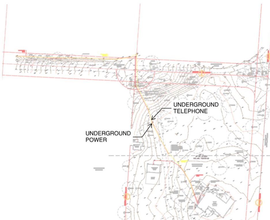
Figure 2: Site Underground Power and Communication
