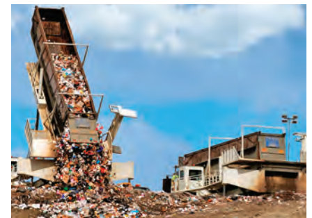
Tippers unloading transfer trailers at landfill
