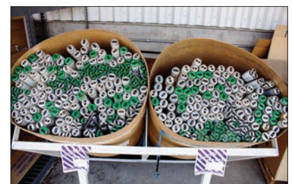
Fluorescent lights and other mercury-containing bulbs and tubes are collected as hazardous waste
