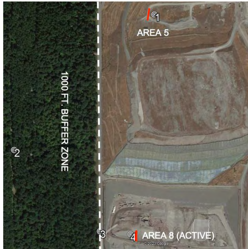
Figure 3-2. Image of vibration monitoring layout. Red lines represent locations where vibratory rollers were used to take vibration measurements. Modified from: QSI 2020b.
