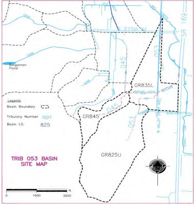
The area was split into three basins GR825U, which is the upper basin, GR835L, which is the lower green river flood plain area of the basin and GR845 which is the area shown draining to Trib 045 which ties into Trib 053 via the Venture ditch. The basin land-use perland data can be found in the March 2008 *Mill Creek Tributary 053 Hydrologic and Hydraulic Analysis RM 0.0 to RM 1.2 Study*. The following table shows the summary KCRTs output for each of the sub-catchments from the 2008 Study:
