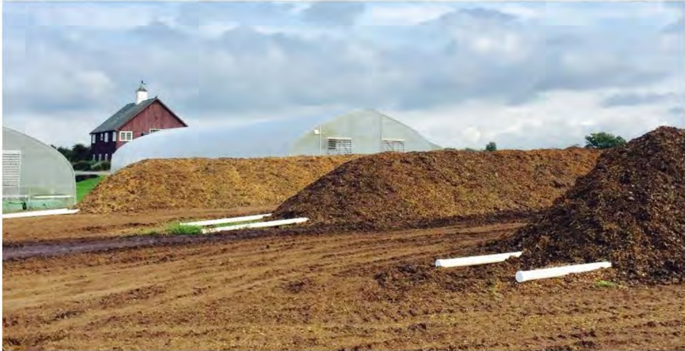
ASP system with pipe-on-grade positive aeration. Photo courtesy of O2 Compost Technologies
