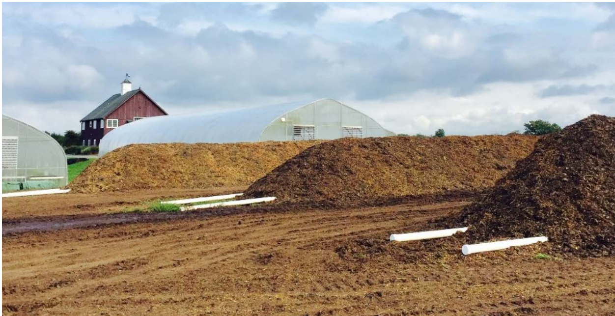
Figure 2. ASP system with pipe-on-grade aeration. Photo courtesy of O2 Compost Technologies.
