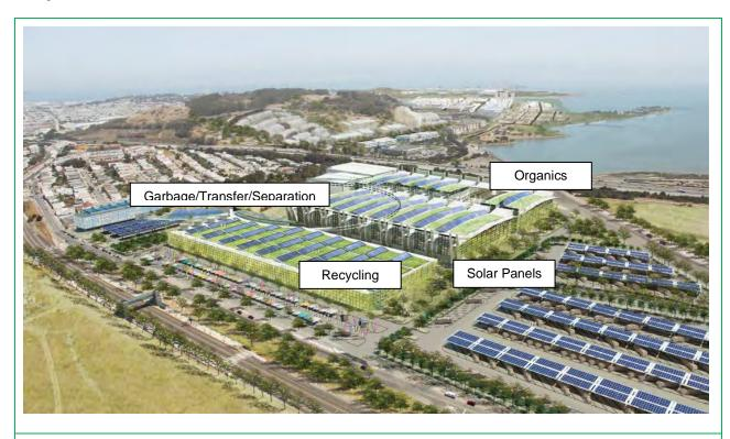
Figure 6. Conceptual Design for San Francisco Zero Waste Facility
