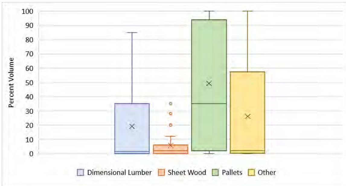
Figure 17. Composition by Volume of Inbound Wood Load Samples (n=25) at C&D Processing Facilities
