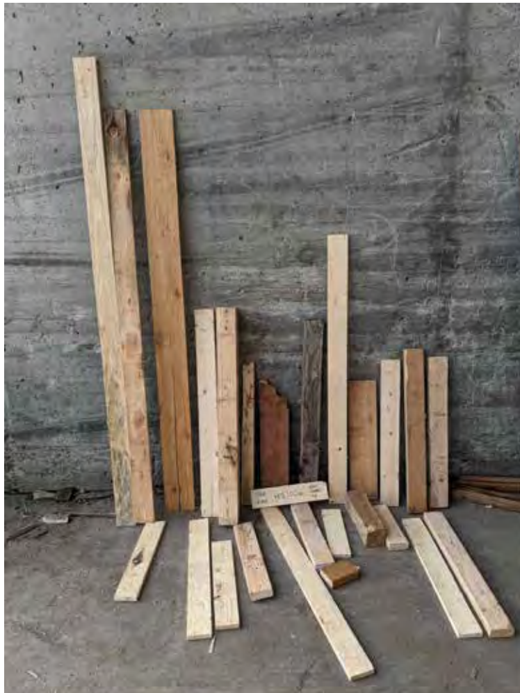
Figure 21. Example of a Hand Sort Sample Consisting of 20 Pieces of Dimensional Lumber
