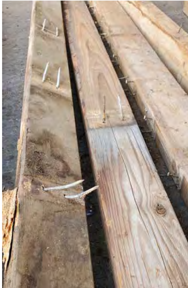
Figure 27. Example of Long Dimensional Lumber with Few Usable Sections of 6 Inches or Longer, Due to Nails
