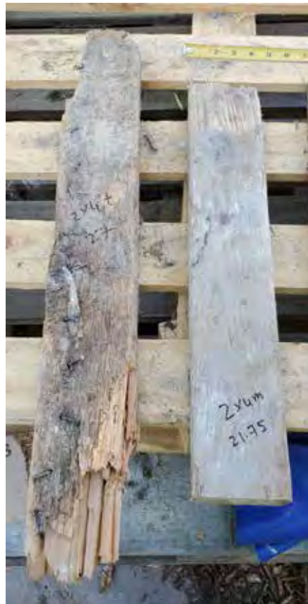
Figure 23. Examples Showing Variance in Dimensions of 2x4s (true on left, modern on right)
