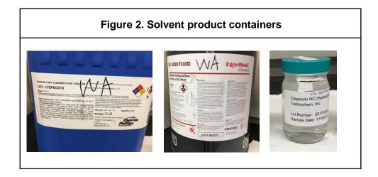
Solvents in 5-gallon product containers were transferred to pre-cleaned 40-mL capacity Volatile Organic Analysis (VOA) vials and 250-mL capacity I-CHEM jars (I-CHEM #220-0250) using a 100-mL capacity disposable serological pipette. The 250-mL product containers provided by Technichem, Inc. were delivered directly to the King County Environmental Laboratory (KCEL). All sample containers were delivered to KCEL at room temperature.
