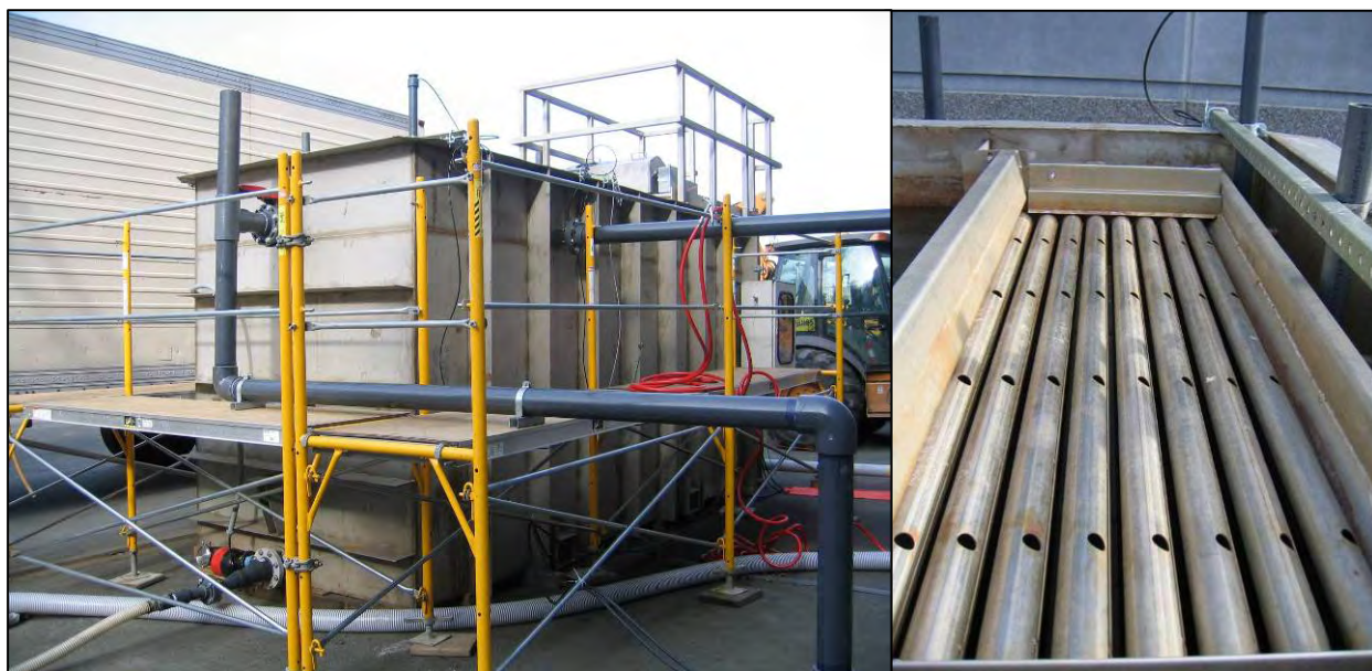
Figure 5-2. Exterior of the CSO Treatment Pilot Plant (Left) and Lamella Plates (Right)
