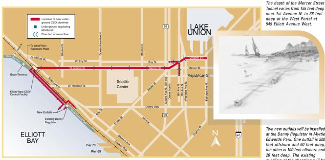
at the Denny Regulator in Myrtle Edwards Park. One outfall is 500 feet offshore and 60 feet deen the other is 100 feet offshore and overflow at the shoreline will be removed.
