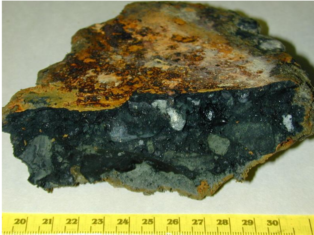
Fig. 13: Close-up of one half of sample #4. Note, the rocks in the corrosion scale.
