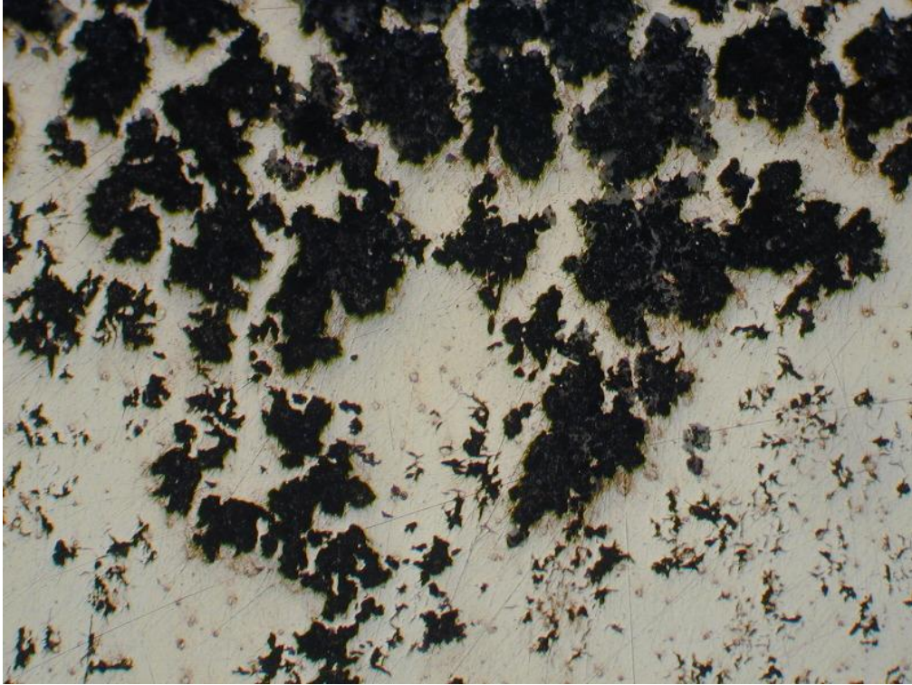
Fig. 35: 100x view of Fig. 33 at the deepest area of corrosion.
