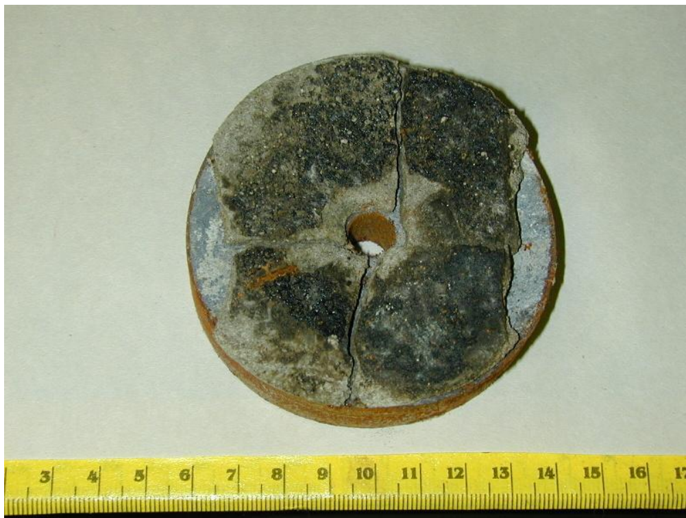
Fig. 4: Overall view of the ID of sample #2. Note, the tar (asphalt) coated concrete was retained with this sample.
