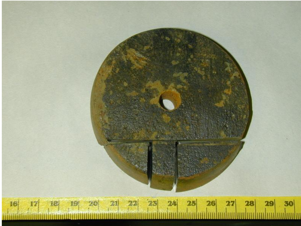
Fig. 17: Overall view of sample #1 after sectioning for metallurgical examination.
