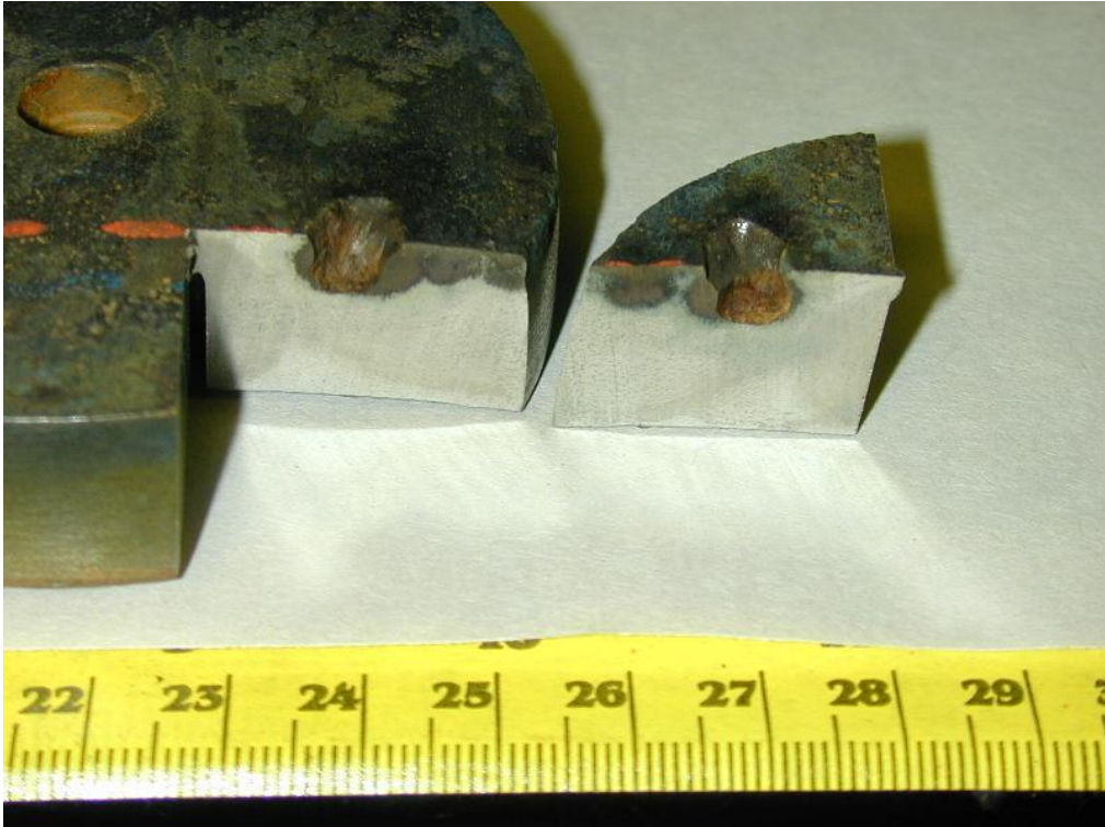
Fig. 22: Cross-sectional view of the pitting and graphitic corrosion.
