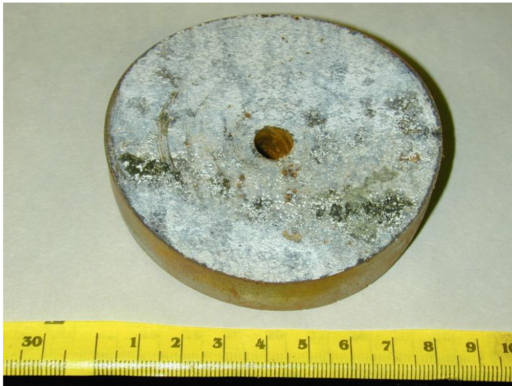
Fig. 2: Overall view of the ID of sample #1. Note, the white material is residue from the concrete liner.
