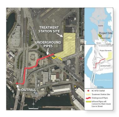
Construction of the facility, related pipes and outfall structure will reduce the amount of untreated rain and wastewater currently entering the Duwamish River by 95%. Outfall construction is expected to begin early this summer and be complete by Spring 2019. The treatment station is expected to open in early 2023.
