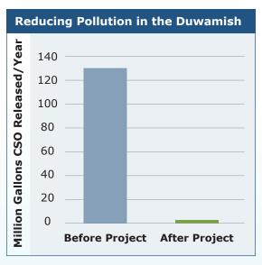
In Georgetown, King County will build a wet weather treatment station to help protect the Duwamish River from CSOs. During heavy rainstorms, the new station will clean excess sewage and stormwater before it enters the Duwamish River. The new facility will reduce the amount of untreated wastewater entering the Duwamish by 95%.
