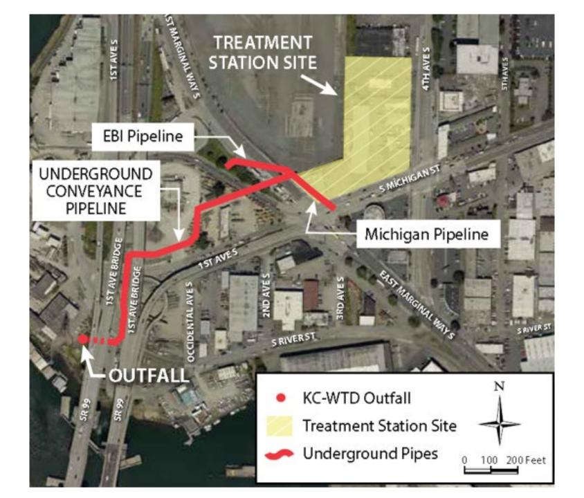
When built, the treatment station will collect and clean up to 70 million gallons of sewage and storm water per day before safely releasing it into the Duwamish River.
