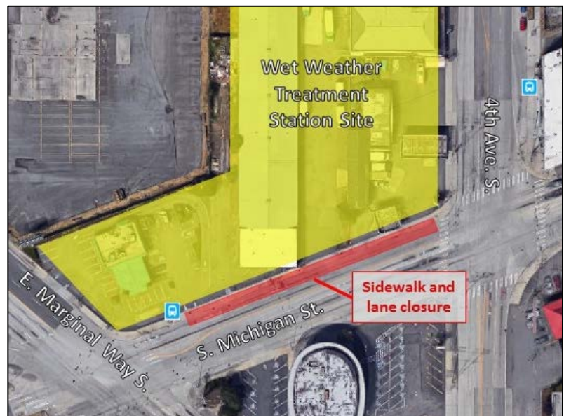
Location of sidewalk and lane closure along S. Michigan St.
