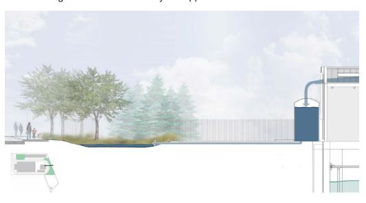
Drains from rooftops attach to cisterns which collect and store rainwater so it can be used later on vegetation. Collecting rainwater has the additional benefit of reducing the amount of water that enters the storm sewer systems and treatment facility. This process helps to lower costs, energy, and resources needed to manage and clean stormwater. The image on the left shows how the cisterns will function once installed.
