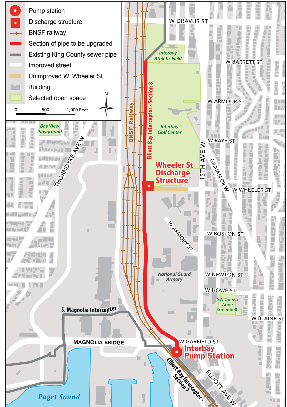
King County plans to upgrade a nearly one-mile section of pipe in the Interbay neighborhood.
