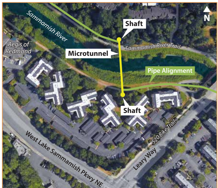
Approximate shaft and microtunnel locations.
