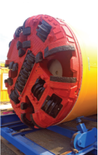
We will use microtunneling to cross under the Sammamish River.
