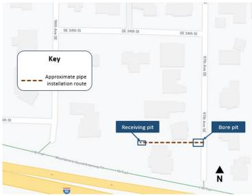
The red dotted line marks the approximate path the pipe will take during trenchless pipe installation.
