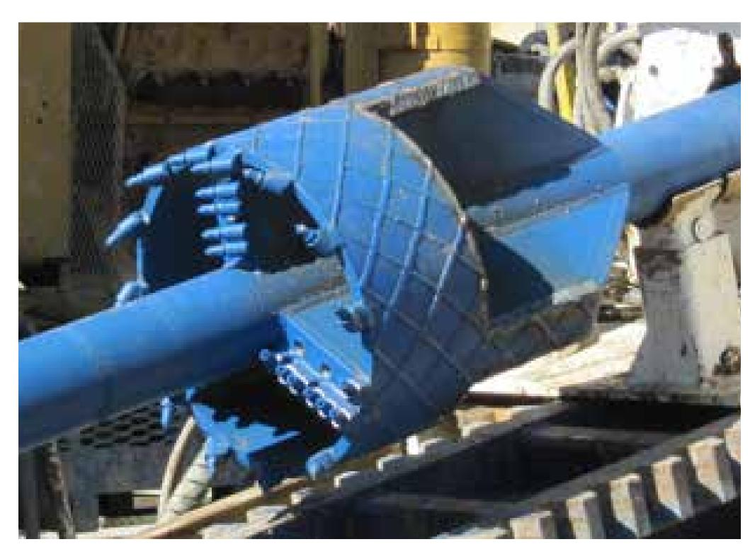
Crews install the new pipeline using special equipment that drills a small hole along the future pipe route. There is a wire on the surface that tracks the location of the drilling equipment underground (above, left). Crews enlarge the hole using equipment called reamers (above, right) until it is large enough for the new pipe. A special type of mud is used to keep the hole open until the pipe is pulled into place.
