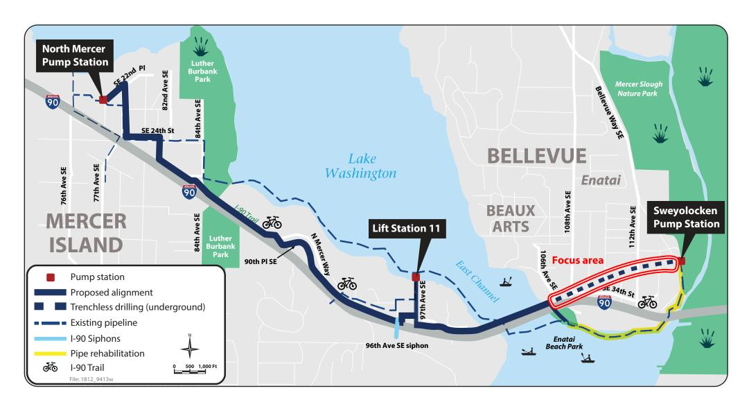
In order to increase capacity in our sewer pipes, this project includes the installation of a new sewer pipe under the Enatai hillside from Enatai Beach Park to the Sweyolocken Pump Station.
