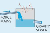
wastewater splashes into a structure where it will be transferred to a non-pressurized pipe that carries the sewage by gravity.
