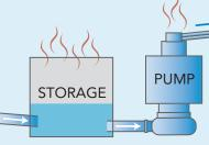
At pump stations, gases are released as sewage is churned through mechanical pumps.
