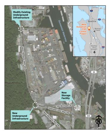
more than one overflow per year on average. To accomplish this, King County is designing a storage tank near the 1st Avenue bridge. The storage tank will hold stormwater and wastewater during large storms, which will reduce risk of raw sewage from overflowing into the Duwamish River. After the storm, the water will flow to West Point Treatment Plant for cleaning.
