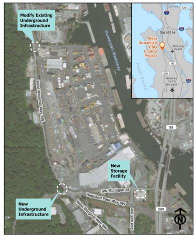
Park drainage basin into the Duwamish River to no more than one overflow per year on average. To accomplish this, King County is designing a storage facility near the 1st Avenue bridge. The storage tank will hold stormwater and wastewater during large storms, which will reduce the risk of raw sewage from overflowing into the Duwamish River. After the storm, the water will flow to West Point Treatment Plant for cleaning.
