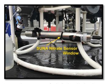
**Figure 6.** Washington State Dept. of Ecology's Submersible Ultraviolet Nitrate Analyzer (SUNA) pictured above attached to King County's water sample carousel frame. This new instrument rapidly measures changes in nitrate as the carousel is lowered through the water, and was recently added to provide more information on nutrient dynamics.
