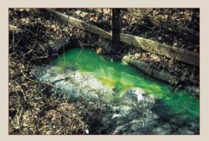
**Dye Testing** involves pouring non-toxic fluorescent colored dye down roof drains or catch basins to see if that dye makes its way into the sewer.
