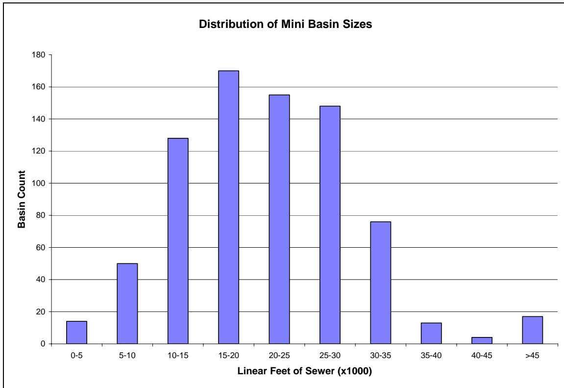
Figure C1 Distribution of Mini Basin Sizes (x 1,000 LF of Sewer)
