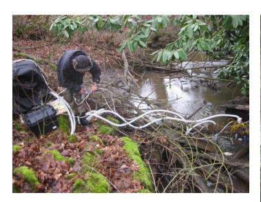
The sampling unit consists of a DC-powered bilge pump connected to a frame which supports two parallel filtration housings and batteries. Stream water is pumped through the filtration housing units, each equipped with a 20-inch long, 4-inch diameter filter bag. All bags are made of 5 micron polypropylene felt, pressure rated to 15 psi.
