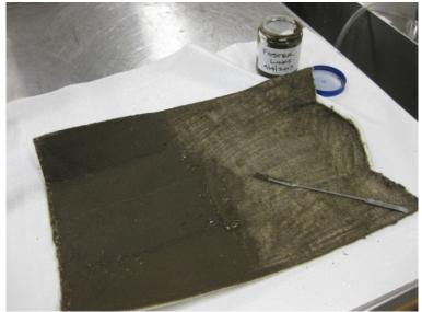
Filters are cut open and solids carefully removed. Filters do not capture all suspended solids and removal of solids from filters can not collect all material on filter.
