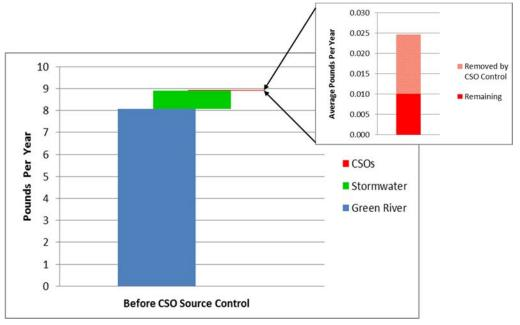
Figure 4. Estimated Relative PCB Inputs to the LDW Before and After CSO Control
