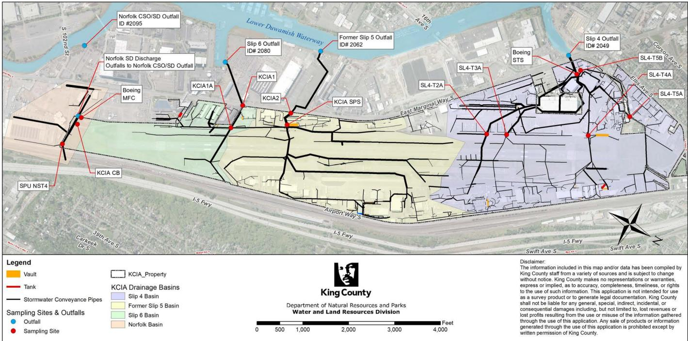
Figure 6. KCIA Stormwater Basins and Source Tracing Sampling Locations
