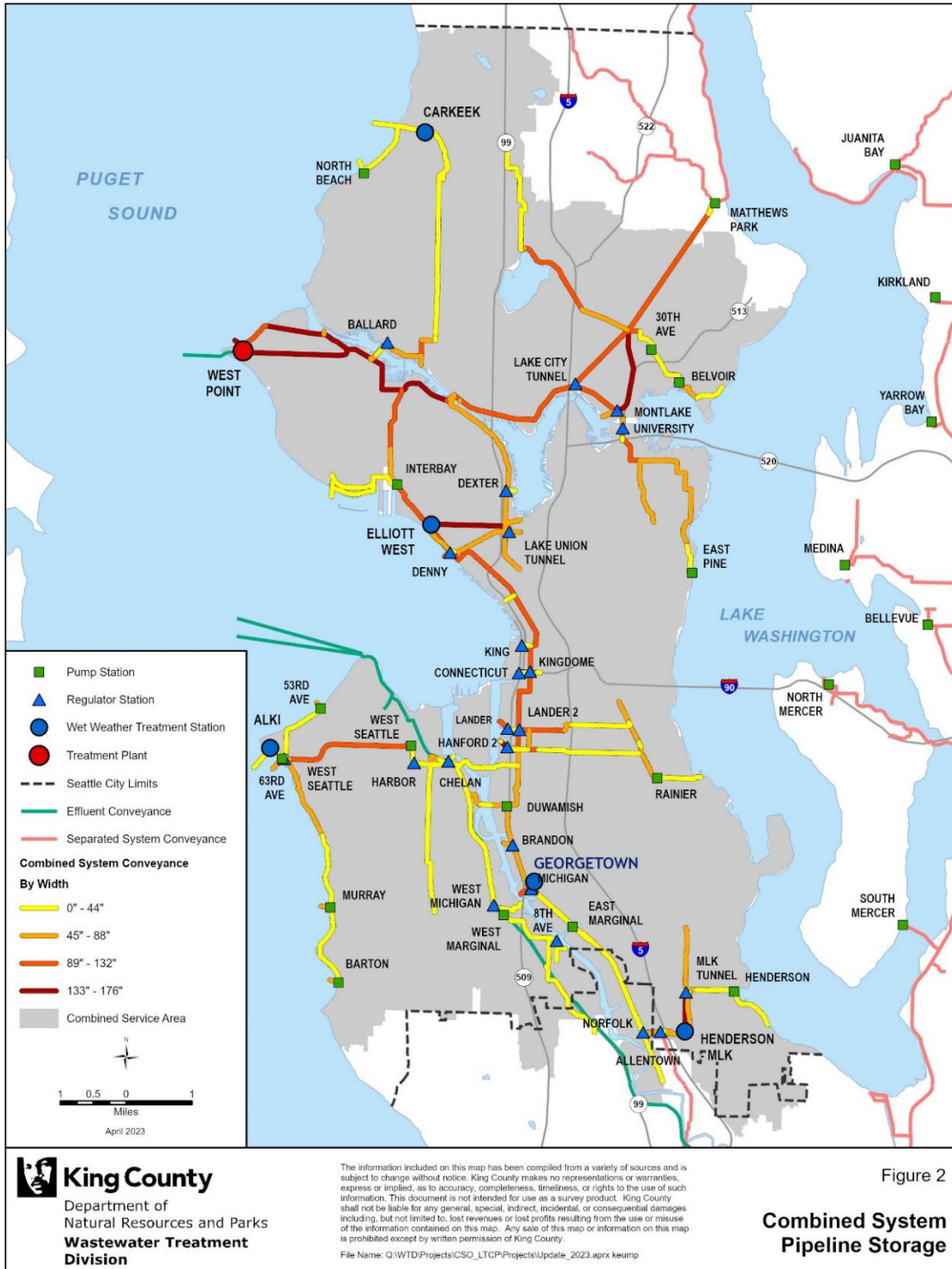
Figure 2. King County Wastewater West System Pipeline Storage
