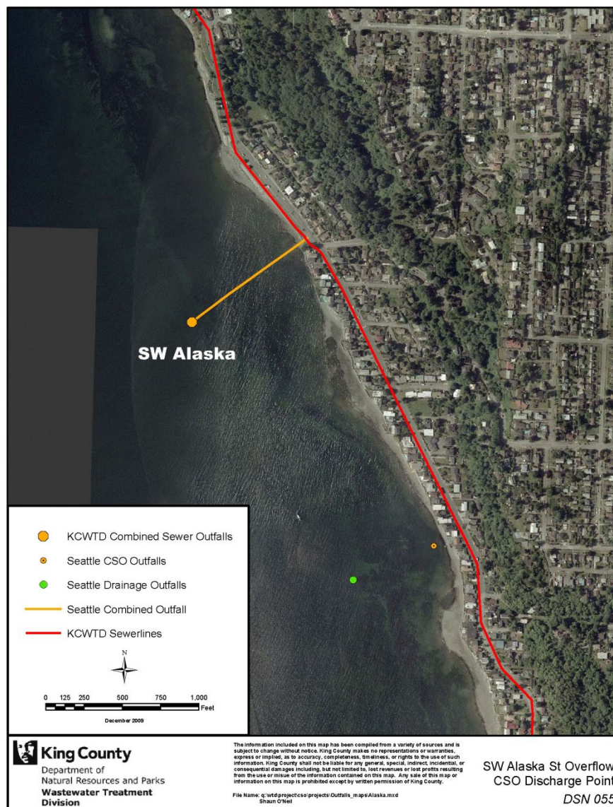
Figure 2-14. Southwest Alaska Street CSO Discharge Point
