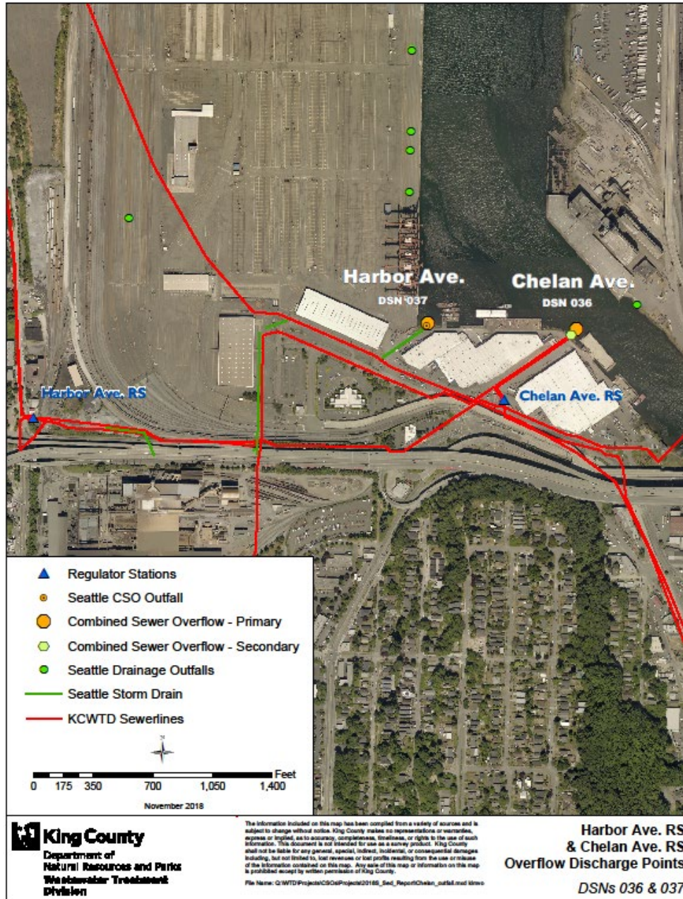
Figure 4-11. Harbor Avenue Regulator Station CSO Discharge Point
