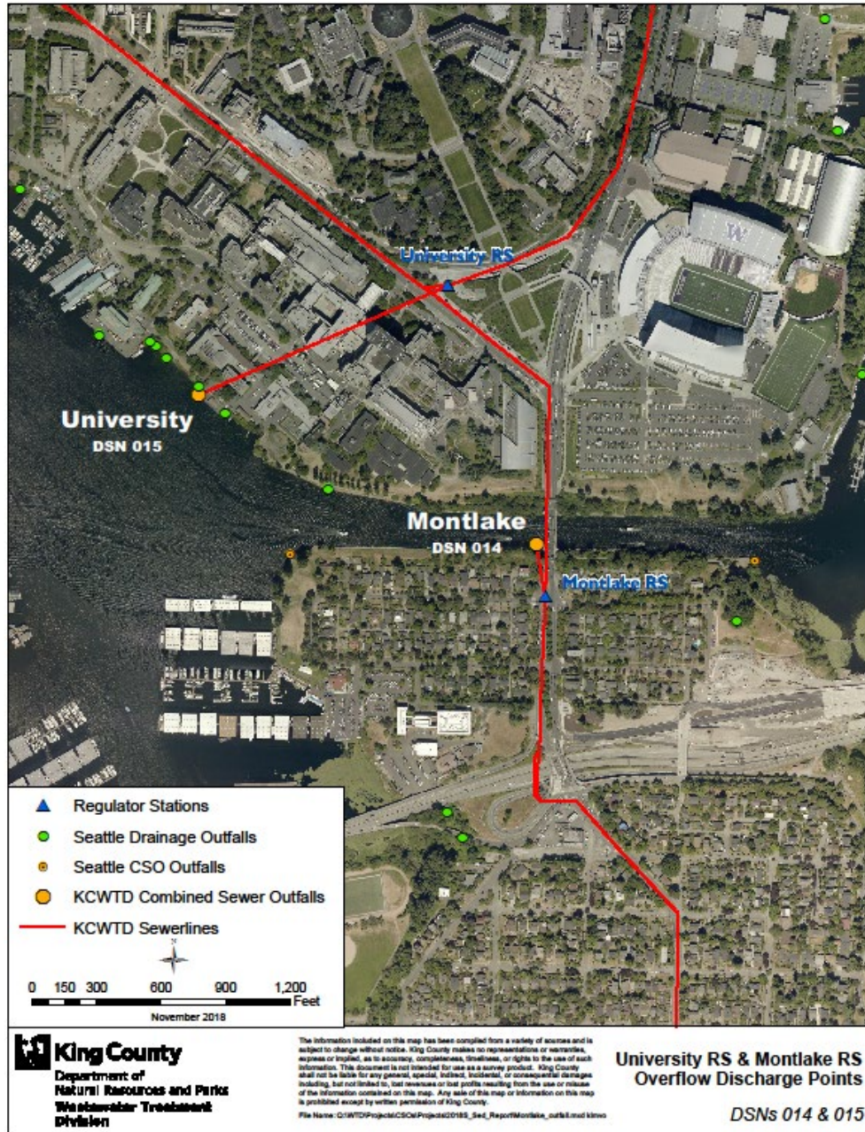
Figure 5-12. University and Montlake CSOs Discharge Points
