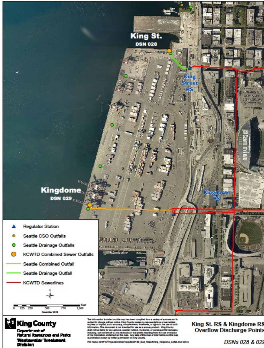
Figure 3-6. Kingdome (Connecticut Street) Regulator Station CSO Discharge Point
