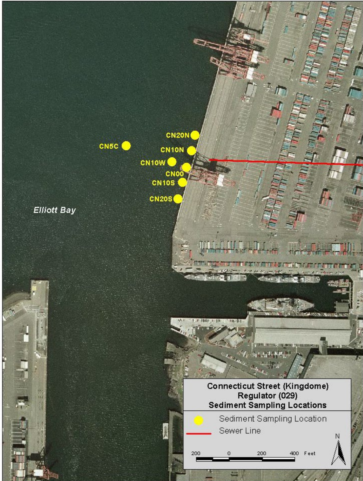
Figure 3-7. Kingdome (Connecticut Street) Regulator Station (029) Sediment Sampling Locations
