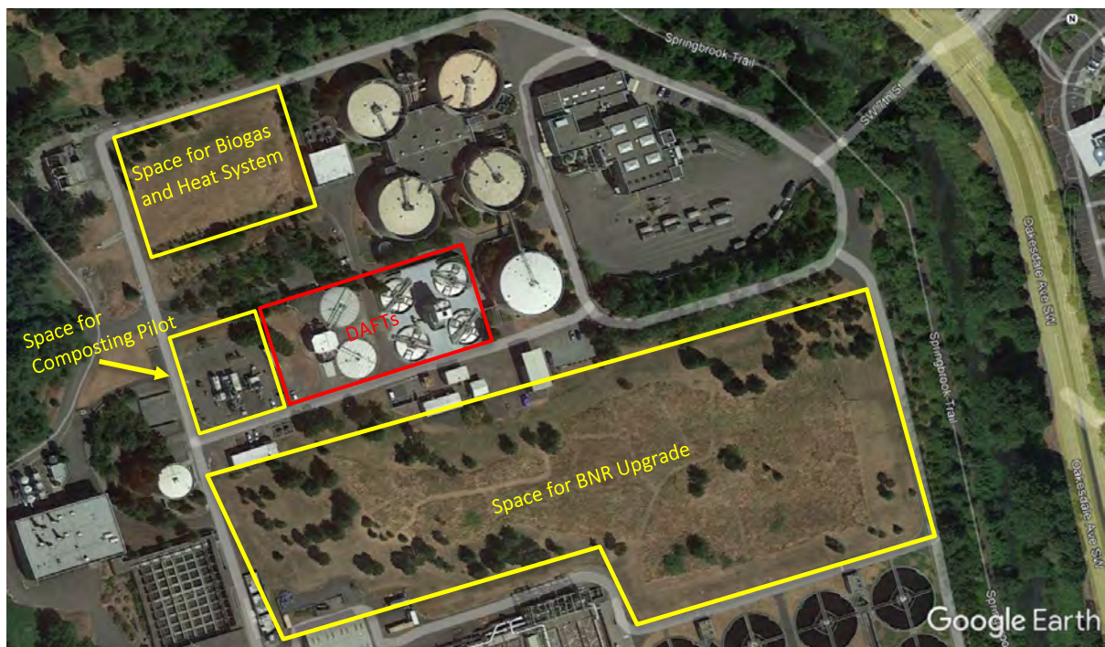
Figure 2. Site Plan of South Plant Showing DAFT and Spaces for Future Use
