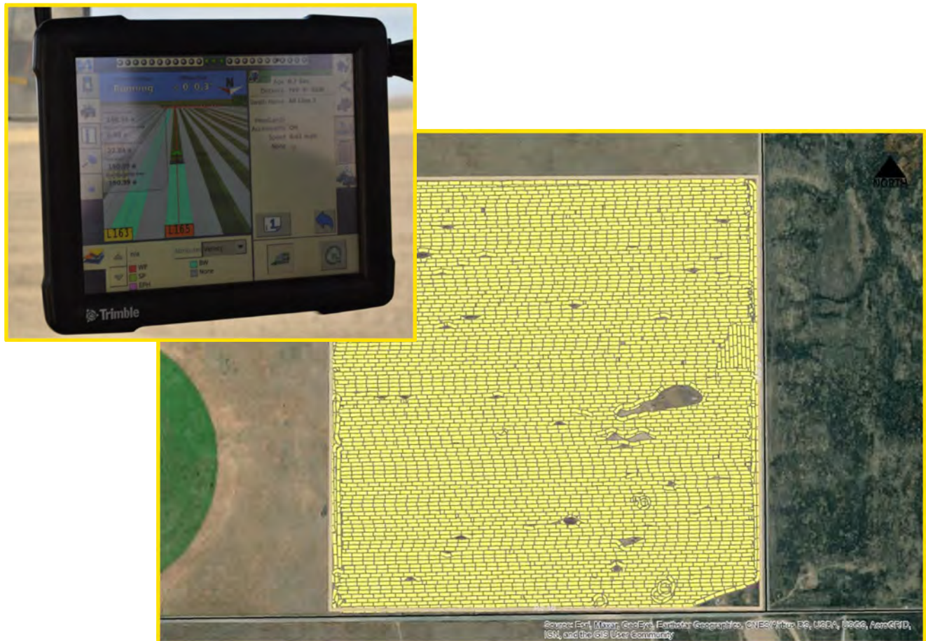
A Trimble GPS display shows the application path of a tractor applying biosolids (top left); A map created by exporting data captured by GPS and imported to Geographic Information Systems showing the final application of a project site (above).
