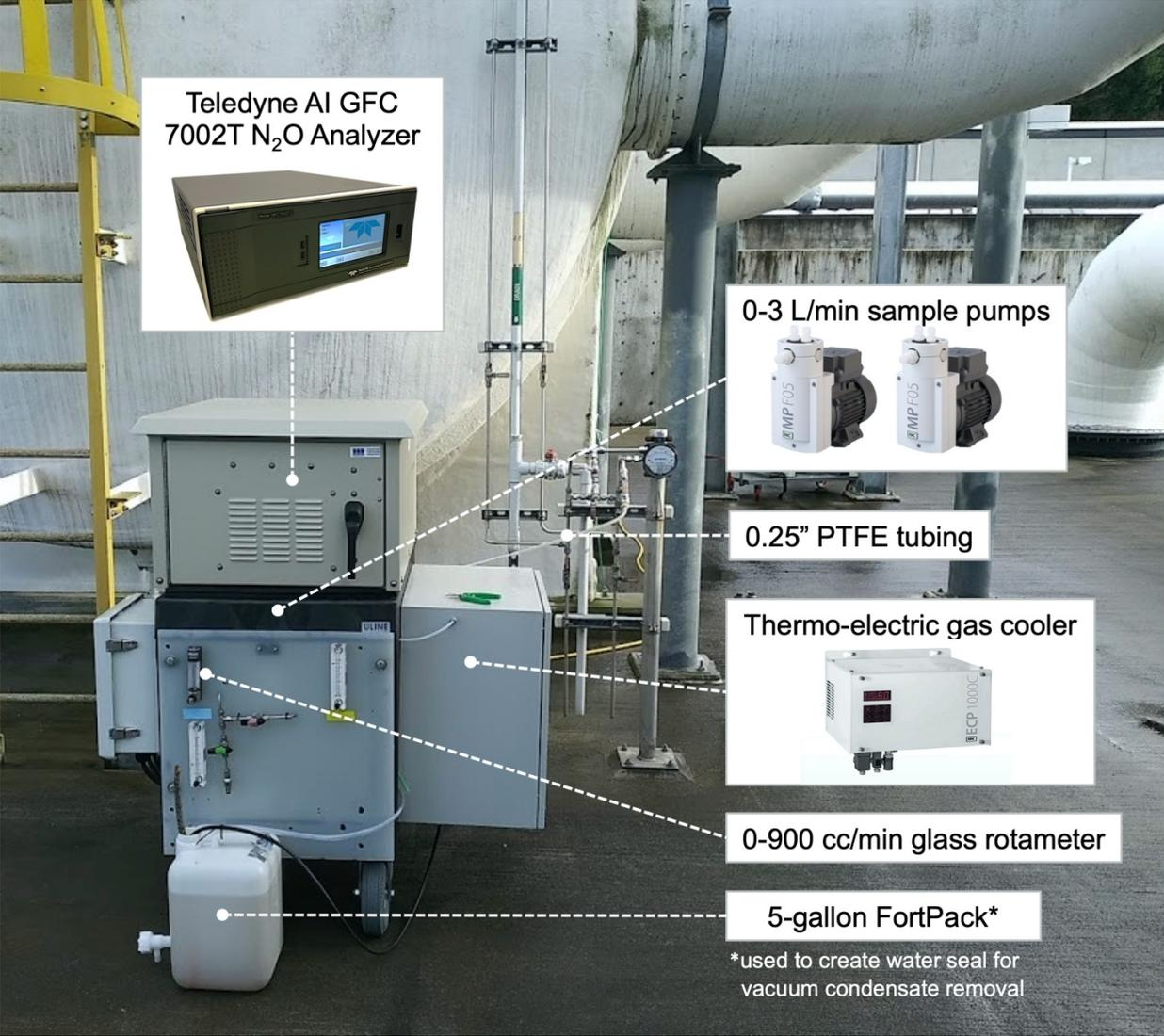
Figure A5. Gaseous N<sub>2</sub>O field sampling unit.
