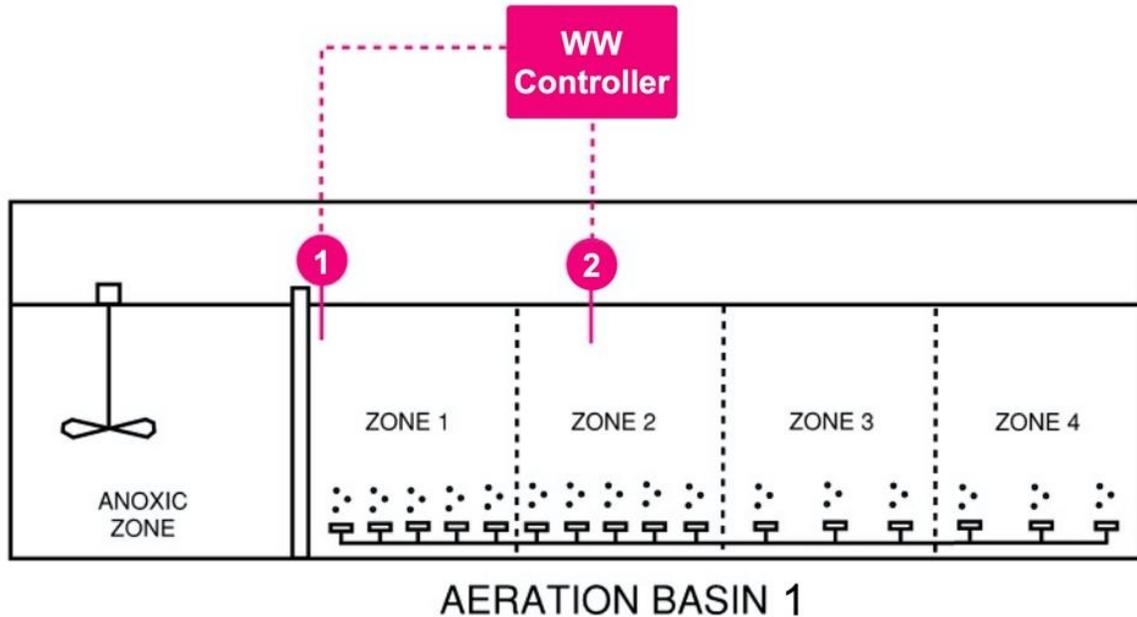
Figure 3-3. Aqueous N<sub>2</sub>O measurement setup. N<sub>2</sub>O sensors are labeled 1 and 2.
