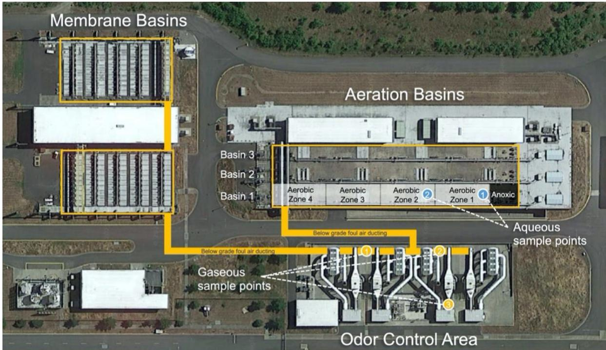
Figure 3-2. Brightwater Treatment Plant with N<sub>2</sub>O monitoring configuration.
