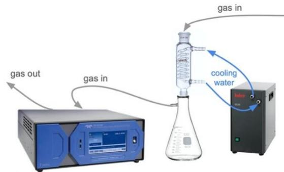
Figure B3. N<sub>2</sub>O analyzer and condenser setup
