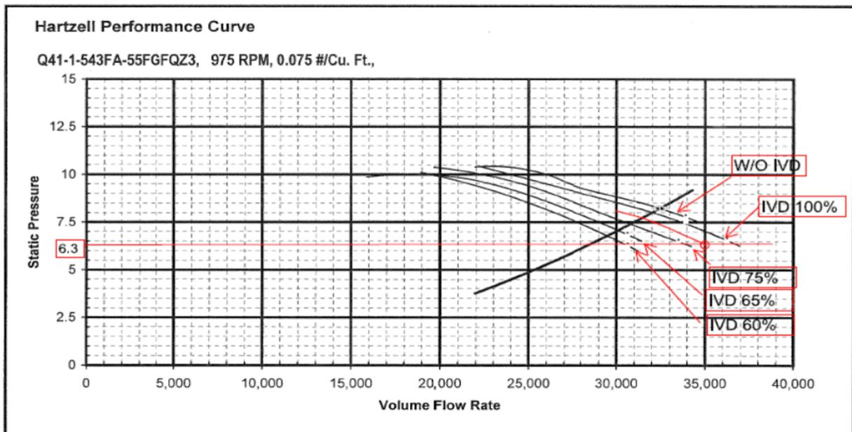
Figure A6. Performance curves for Brightwater odor control blowers. Static pressure is reported in inches water column (in wc). Volume flow rate is reported in standard cubic feet per minute (SCFM). IVD stands for Inlet Vane Damper and is reported as percent open.
