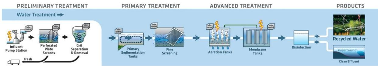
Figure 3-1. Brightwater liquid stream treatment process (King County, 2018)<sup>83</sup>.
