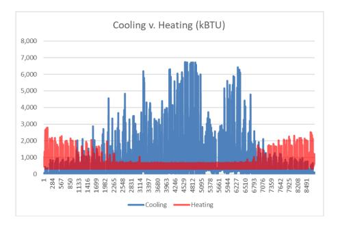
Figure 3 Mixed-Use Building Hourly Cooling/Heating/DHW Loads
