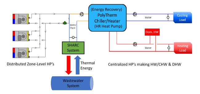
Figure 1 Example of a Building with Internal Energy Recovery
