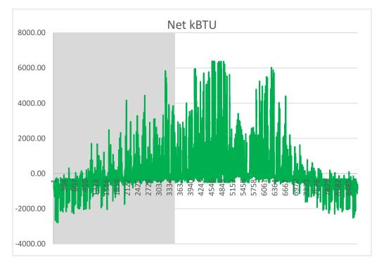
Figure 5 Mixed-Use Building Hourly Plot of Net Cooling/Heating/DHW Loads
