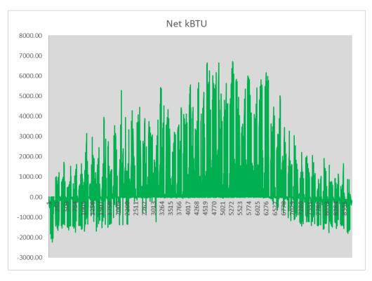
Figure 4 Office Building Hourly Plot of Net Cooling/Heating/DHW Loads
