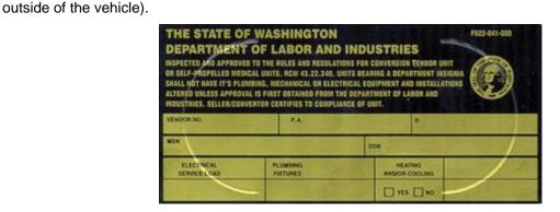
body and frame design and the installation of plumbing, heating and electrical equipment. Contact the L&I Plans Examiner at (360) 902-5222 in Olympia for your packet of information on L&I plan review. Obtain L&I inspection and seal of approval prior to your plan review by the Health Department (black label affixed to the
